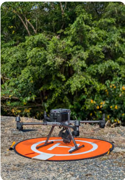
DJI Matrice 350 RTK drone equipped with a Zenmuse H30T thermal infrared payload used for capturing aerial thermal imagery of roosting spectacled flying-foxes ( Pteropus conspicillatus ). Image: Emmeline Norris.
