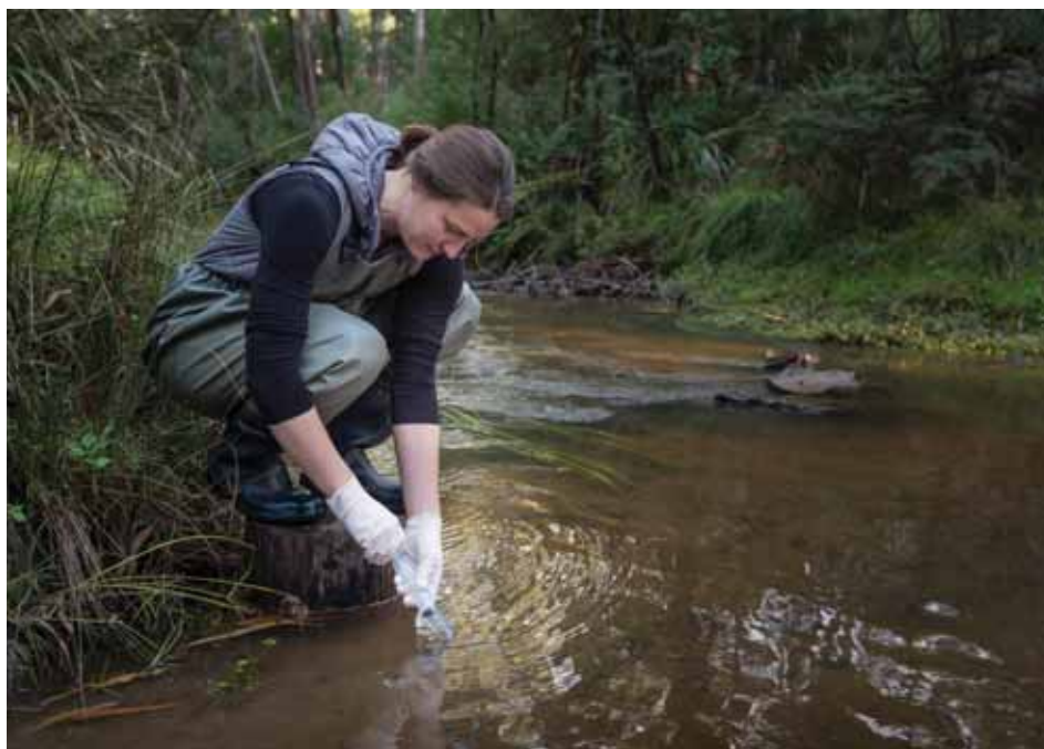
Sampling the waters for eDNA testing. The first part of looking for environmental DNA is collecting a water sample. Here, Lisa Kirkland, a member of the research team for EnviroDNA, draws up a sample of water in a syringe. This water is extracted, then filtered through a 0.22 micron filter on site, then sent to the lab for DNA extraction and analysis. This sample will then be refrigerated and transported to the laboratory for analysis.
